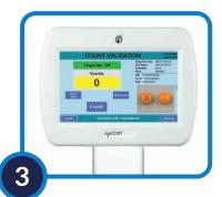
**Verify** - The Eyecon will proceed to count mode if the Rx label matches the stock bottle. The Eyecon will display an error if a mismatch is detected.
