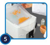
**Dispense** - Press the Finish button to record the transaction. Then lift platter to slide pills into funnel.
