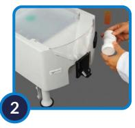
**Scan Bottle** - Scan barcode on stock bottle to validate that you've pulled the correct medication or be alerted to a generic substitution.
